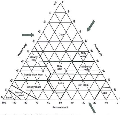
Determine the soil type for the following soil compositions:
